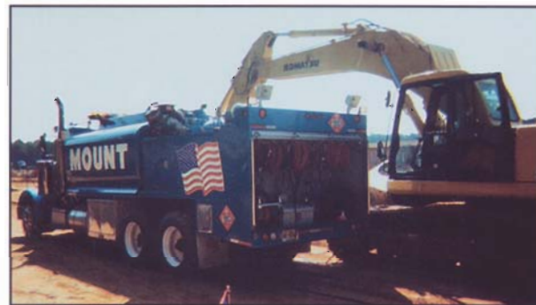
To keep its large fleet up and running, the company stresses good equipment preventive maintenance practices, like investing in field service and lube trucks.
