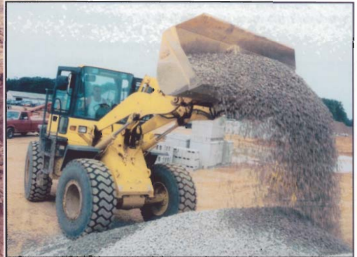
Crews from Mount Construction used a large fleet of Komatsu equipment on a recent expansion project at Edgewood High School in Berlin, New Jersey. This included (clockwise from above left), the operator of a Komatsu PC400LC-6 excavator cutting a deep utility trench; the operator of a WA250 wheel loader stockpiling aggregate; and the operator of a D61 dozer using the machine's blade for grading.
